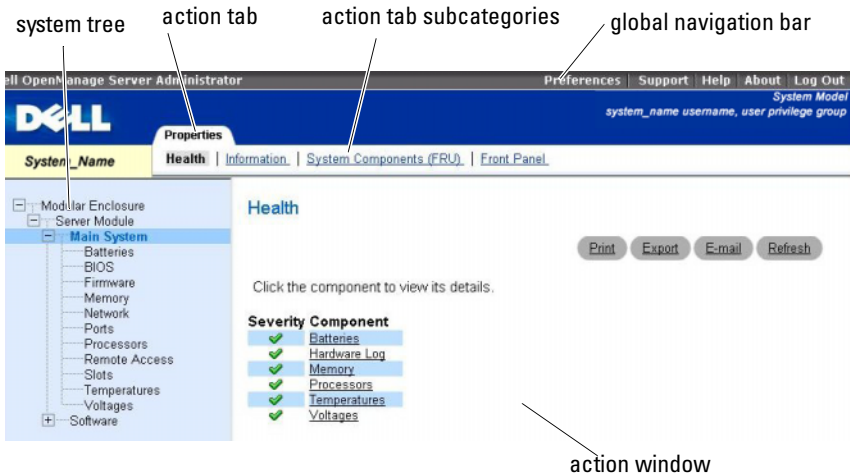
Figure 5-2. Sample Server Administrator Home Page — Modular System
